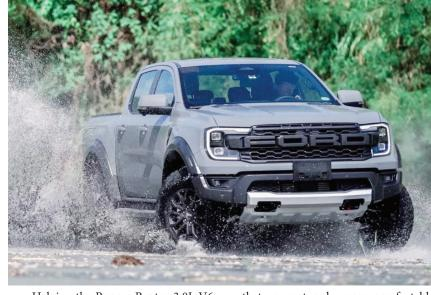
Helping the Ranger Raptor 3.0L V6 handle anything from smooth roads to mud and ruts and everything in between are up to seven selectable drive modes, including the off-road oriented 'Baja' mode for extreme high-speed off-roading.
